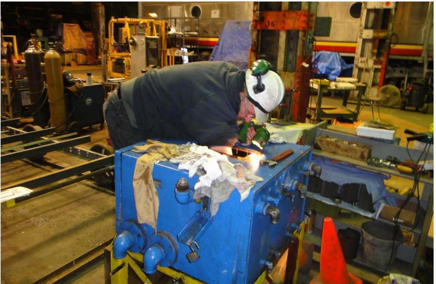
Fred toils to clean out the tie shear's hydraulic tank
